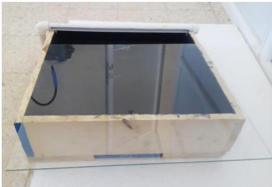
Figure 11: Assemblage of a Solar distiller (Source: Khechekhouché et al., 2020)
